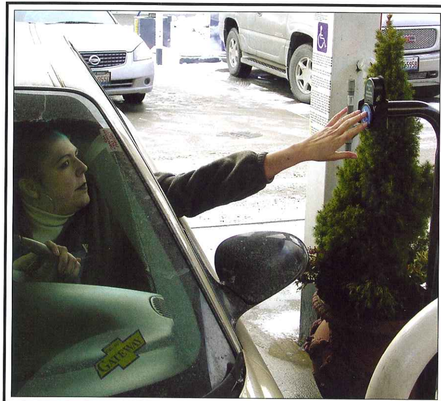
CALL FOR HELP: Drivers in need of fueling assistance can press a FuelCall touchpad that wirelessly transmits to a unit inside the store, thereby alerting an attendant.
